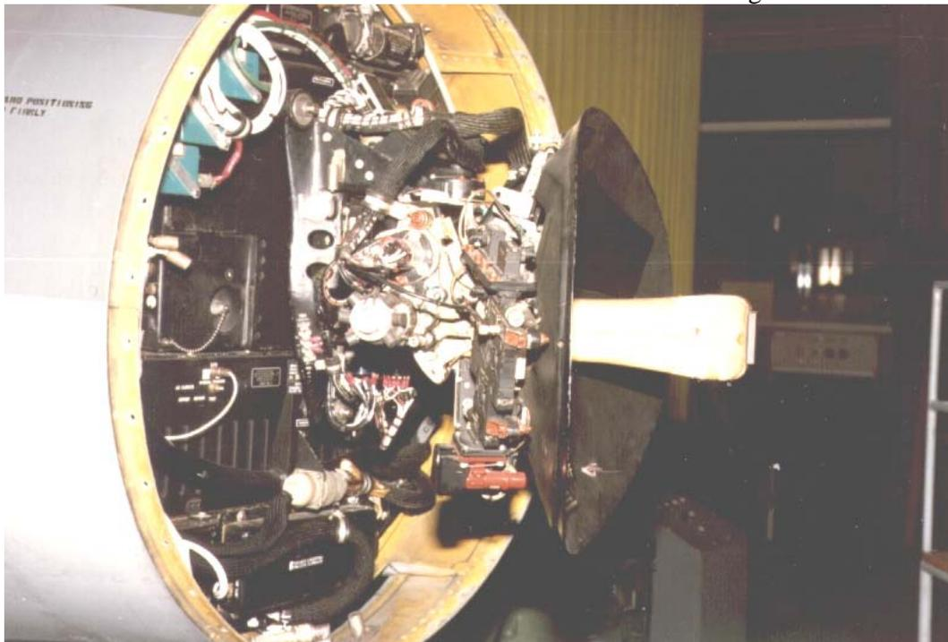
A multi-purpose system consisting of a radar set, that incorporates an optional fire control computer for air-to-air, air-to-ground, and navigation. Used with the fire control computer in air-to-air missions, NASARR figures for the pilot lead angle of attack for automatic rocket releases, and lead angle of attack (with information supplied to the director gunsight) for the M-61 Vulcan gun.
